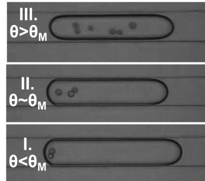
Fig. 4: Particle concentration profiles in a microchannel with 200x100 $\mu\text{m}$  cross section. High efficiency particle concentration occurs when  $\theta < \theta_M$ , and mixing occurs when  $\theta > \theta_M$ .
