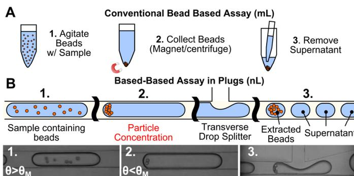
Fig. 1: Comparison of bead based assays in the traditional vs. plug format. The latter is achieved by field-free particle concentration followed by transverse drop splitting.
