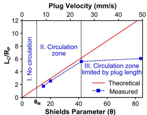
Fig 5: Theoretical and measured lengths of the particle circulation zone graphed vs. the Shields number, which scales with plug velocity. The dotted lines demarcate the 3 flow regimes.
