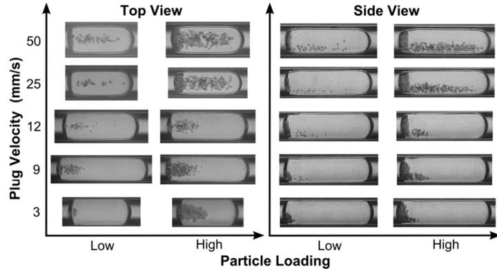
Fig. 3: Particle concentration profiles in a 500  $\mu\text{m}$  ID circular channel. Both the top and side view are shown [8].
