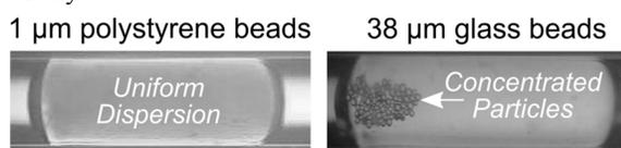
**Fig 6:** Top view comparison of experimental concentration profiles with small, light particles versus large, heavy particles at an identical flow rate of 3 mm/s in a 500  $\mu\text{m}$  diameter circular channel. Both experiments use a high particle loading of  $>10^5/\text{mL}$ .
