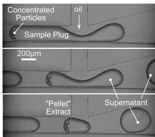
**Fig. 7:** Bead extraction using a transverse drop splitter. The last daughter droplet contains the concentrated particles.
