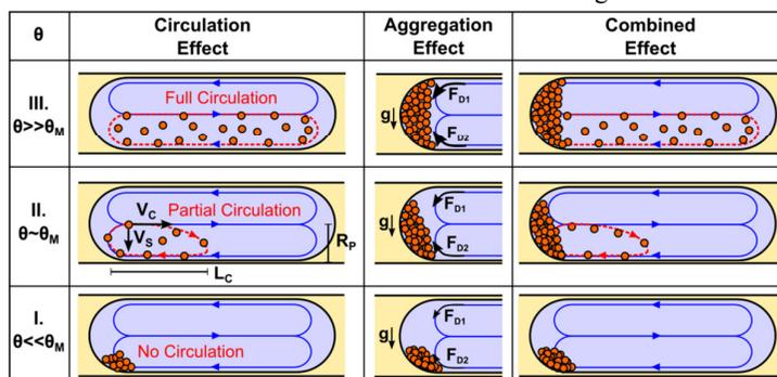
Fig. 2: Theoretical model of particle concentration in plugs (Side View). Three flow regimes are described by the Shields number  $\theta$  (column 1). In each regime, the circulation effect and the aggregation effect are illustrated in columns 2 and 3, respectively. The combined effect is shown in column 4.
