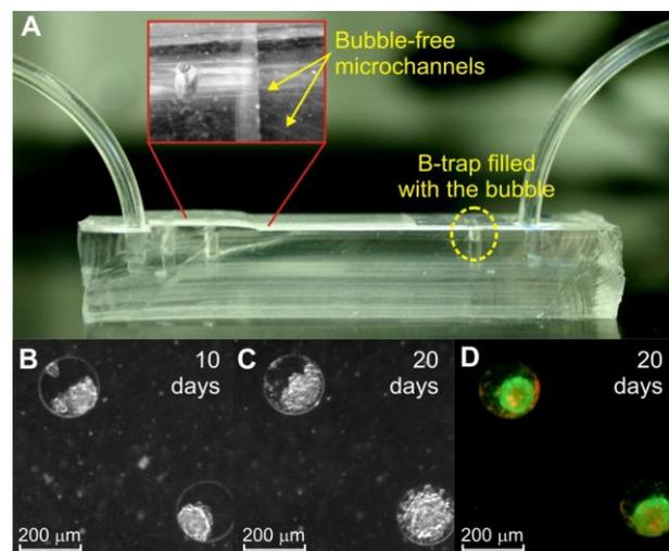
Figure 6: (A) Bubble traps integrated with the cell culture microsystem (after stop-flow 24h incubation). (B,C) Growth of correct spheroids. (D) Cell viability assay.
