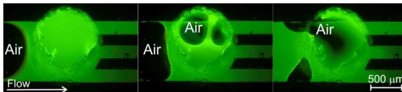
Figure 3: Sequencing frames of the experiment on bubble trapping in the multichannel b-trap.
