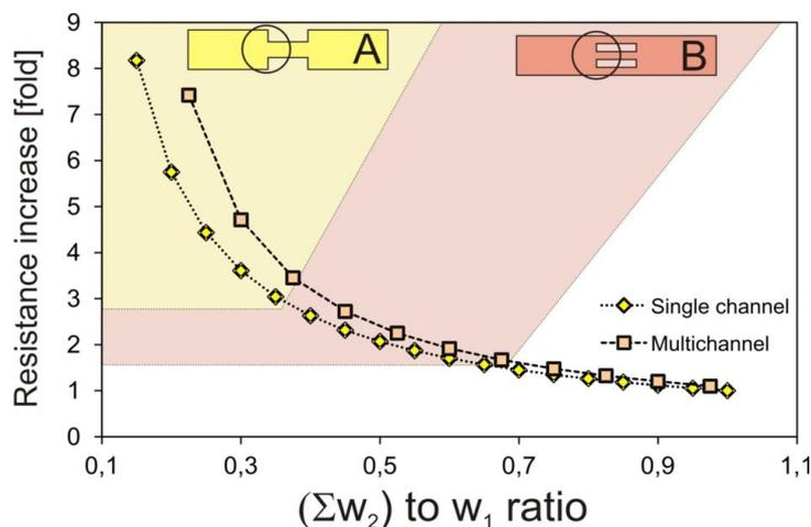
Figure 4: Results of fluidic resistance calculations for different variants of obstacles. Fluidic resistance increase suitable for effective bubble trapping according to experimental results marked for a single channel (A) and multichannel (B) b-traps.
