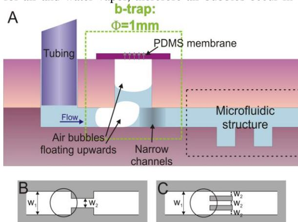
Figure 2: (A) Construction of the b-trap containing PDMS chip: bottom layer contains microfluidic structure and upper layer contains tubing connection ports and b-trap. PDMS membrane was bonded using oxygen plasma treatment. Variants of narrow channels: (B) single channel and (C) multichannel.
