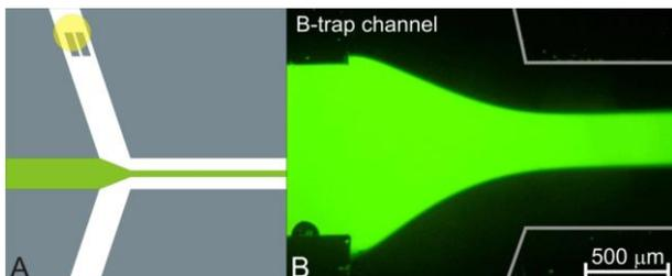
Figure 5: Study of stability of the sheath-flow zone: (A) geometry of the microsystem and (B) symmetrical sheath flow, flow rates at each inlet = 4  $\mu\text{L}/\text{min}$ .
