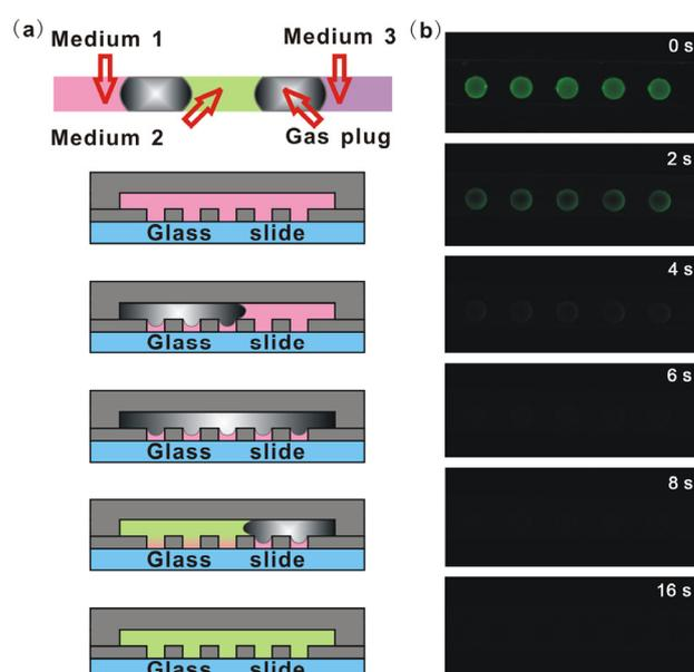
Figure 2. (a) Procedure of switching media from Solution 1 (pink) to Solution 2 (green) by gas-liquid exchange after pre-loading gas-liquid plugs into tubing. Solution 1 (pink) left in the microwells can be completely replaced by Solution 2 (green). (b) A time sequence of optical photographs of the microwells during removal of the fluorescein using a flow rate of 0.5 ml/h at the inlet.
