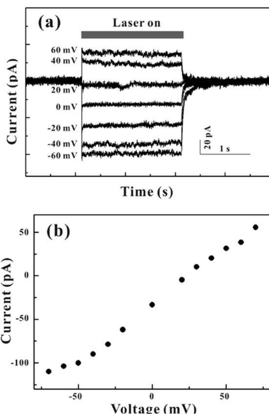
Figure 4: (a) Observed dependence of the laser-gated ion-channel current recordings on the membrane potential. (b) Dependence of the ion-channel current on the applied membrane potential.
