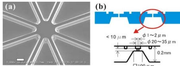
Figure 2: (a) Scanning electron microscope image of the upper Ni mold with cell trapping pattern. Scale bar: 10 μm. (b) Cross sectional structure of the PMMA sensor chip.
