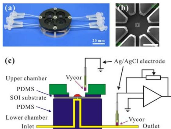
Figure 1: (a) Photograph of 4 channel incubation type planar patch clamp biosensor. (b) Cell trap pattern of PMMA substrate with micropore of 2  $\mu\text{m}$  diameter at the center. (c) Schematic structure of single channel planar patch clamp biosensor.
