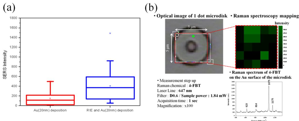
Figure 4. (a) SERS signal intensity of 4-FBT at the bare SiO<sub>2</sub> layer (red) and RIE processed SiO<sub>2</sub> layer (blue)(b) SERS signal mapping data and spectrum of the 4-FBT coded microdisk
