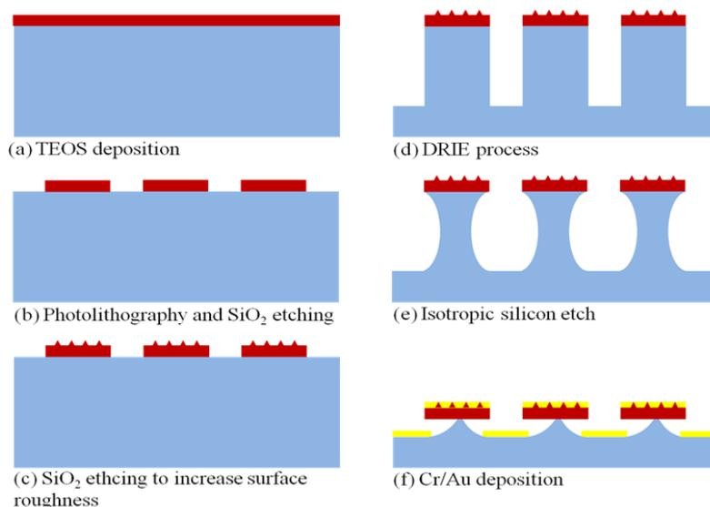
Figure 2. Fabrication process of the microdisk
