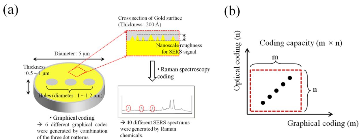
Figure 1. Schematic of the microdisk (a) and the graphical and optical codes map (b)
