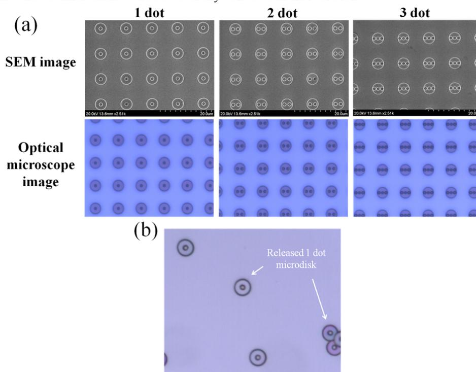
Figure 3. Fabrication results of the microdisk (a) SEM and optical microscope images of the patterned microdisks by photolithography and SiO<sub>2</sub> dry etch (b) The collected microdisks on a slide glass
