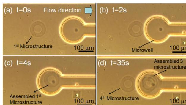
Figure 6. Self-assembly result of microstructures inside microfluidic channel
