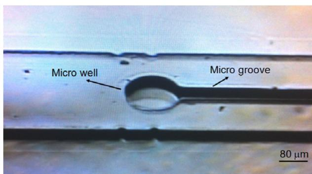
Figure 5. Fabricated bottom part of the PDMS microfluidic device
