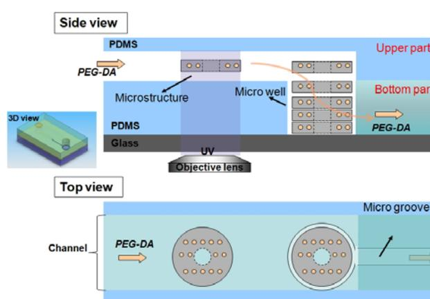
Figure 4. Schematic of a microfluidic device for self-assembly of movable microstructures
