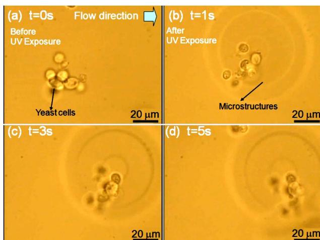
Figure 3. Fabricated movable microstructure embedding yeast cells
