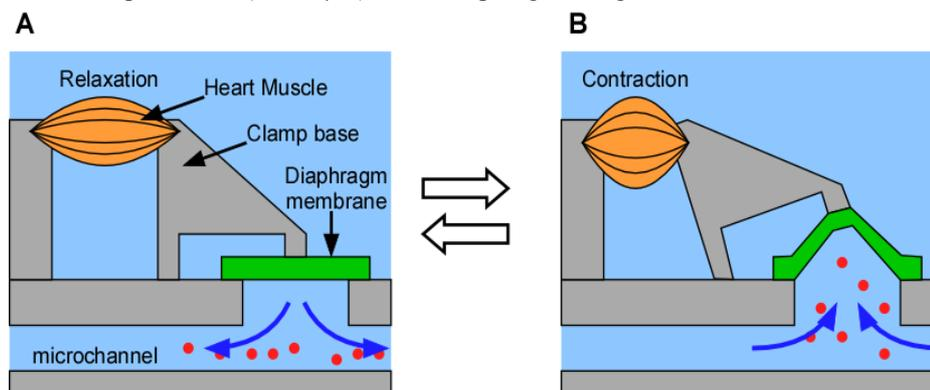
Figure 2. Cross-sectional schematic diagrams of the micropump mechanism driven by contractions of a muscle tissue. The structures are (A) A clamped muscle tissue relaxes in medium. (B) A muscle tissue contracts and then the diaphragm membrane is lifted.
