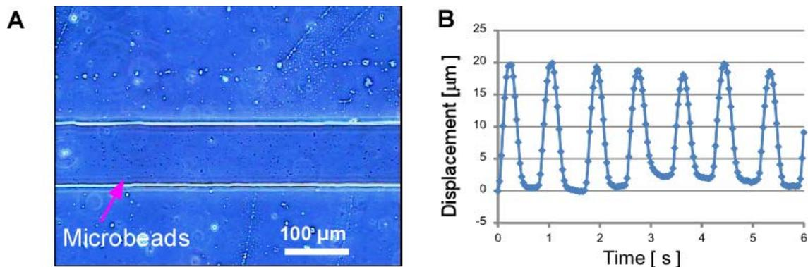
Figure 5. Measurement of pulsation flows driven by the muscle tissue in the microchannel. (A) A microscopic image of flows containing microbeads for the visualization of liquid flow. (B) The displacements of the microbead in the pulsation flows in the microchannel.
