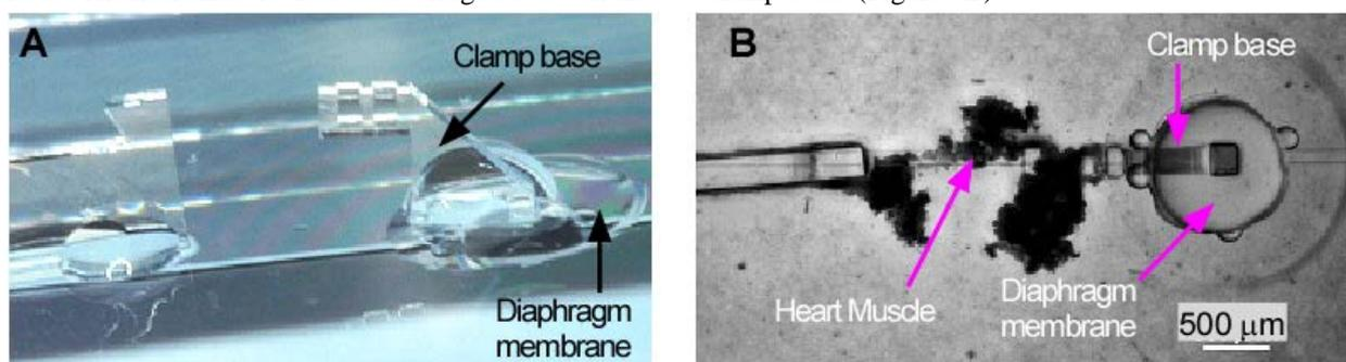
Figure 4. Microscopic images of the clamp base of muscle tissue on the diaphragm membrane. (A) The base without a muscle tissue. (B) A heart muscle tissue of insect clamped with the base.
