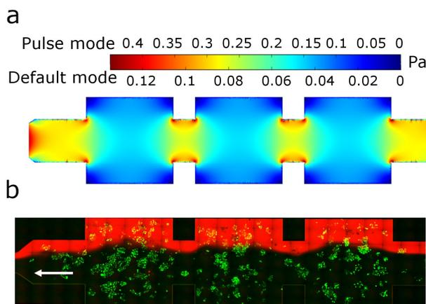
Figure 3: Fluid flow and cell culture in the microfluidic chambers (a) 3D Comsol simulations of the flow shear stress inside the microfluidic chambers during the default and stimulation modes. (b) Fluorescence micrograph showing the GFP-NF- $\kappa$ B tagged HeLa cells (green) cultured in the chambers (around 500 cell per chamber), and the TNF stream (mixed with red fluorescent BSA) operating in the default mode.
