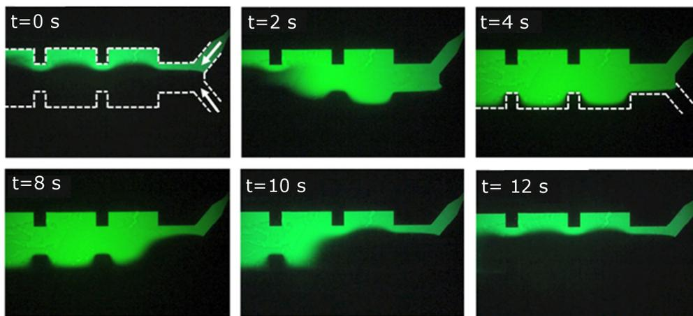
Figure 2: Time-lapse of a 10 s pulse of fluorescein that was added to the TNF reservoir (Figure 1). At  $t=0$  s, the system switched to the stimulation mode by raising the TNF reservoir and then lowered after 8 s back to the default mode. Each chamber has a length side of 2 mm and a depth of  $40\ \mu\text{m}$ .
