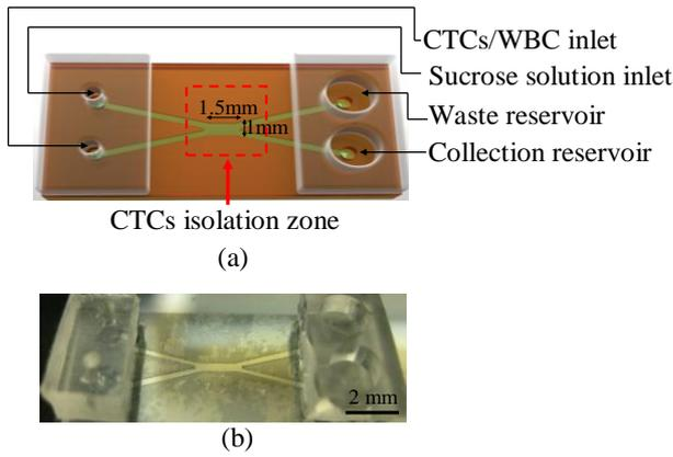
Figure 1: (a) Schematic illustration and (b) a photograph of the microfluidic platform (Top view).
