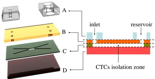
Figure 2: The structure and cross-sectional view of the microfluidic platform.
