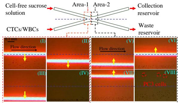
Figure 5: The microscopic images (I-VIII) of the ODEP-based cell (PC3 cells/WBCs mixture) separation process.
