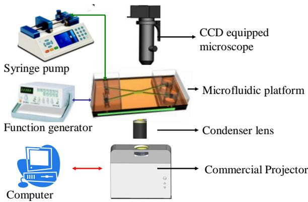
Figure 3: The experimental setup for the ODEP platform.
