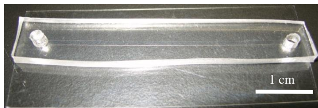
Figure 2. Picture of the microdevice for cell separation. Microchannel height, length and width are 50 \mu\text{m} , 5 cm and 50 \mu\text{m} , respectively.
