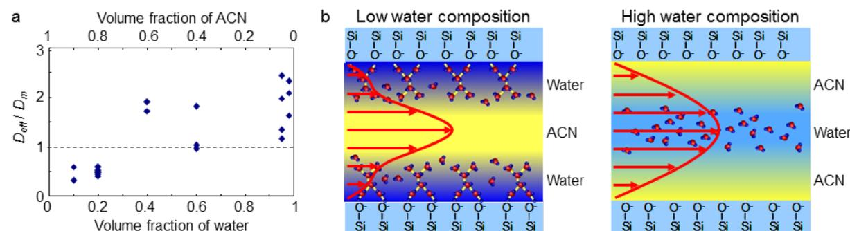
Figure 3. (a) Ratio of diffusion constant in flow ( $D_{eff}$ ) and without flow ( $D_m$ ) plotted against mobile phase composition. (b) Mobile phase partition and suggested flow rate distribution in nanochannel.
