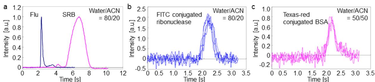
Figure 4. Chromatograms for reversed-phase mode. (a) fluorescein (Flu) and sulforhodamine B (SRB). (b) and (c) fluorescently-labeled proteins.
