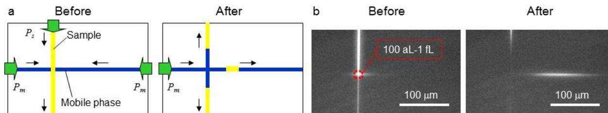
Figure 1. (a) Schematics and (b) fluorescent images of nanochannels before and after injection.
