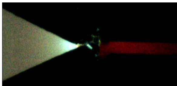
Figure 3. Screen shot showing (on right hand side) the extraction of the red coloured 5(6)-carboxynaphtho fluorescein from a mixture of labeled BSA and free dye (on the left hand side).
