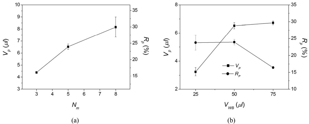
Figure 5. Blood plasma recovery depending on (a) number of membrane and (b) volume of the blood sample.
