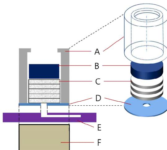
Figure 1. A schematic diagram of the blood filter. A: plastic container; B: permanent magnet; C: filter membrane; D: double-sided tape; E: biochip; F: external control magnet.
