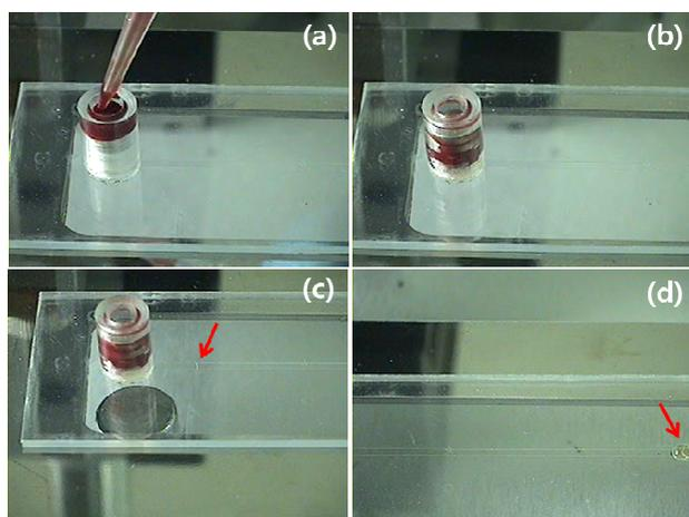
Figure 3. Sequential photos showing the extraction of blood plasma from whole blood. (a) Dropping a blood sample, (b) wetting the membrane, (c) plasma flow into a microchannel by magnetic actuation, (d) collected plasma at the end of the microchannel.
