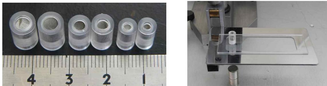
Figure 2. (a) View of the fabricated filter units of different sizes, (b) experimental setup
