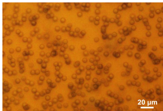
Figure 6. Microscopic images of the fabricated GUVs containing quantum dots (QDs). Highly uniform-sized GUVs were synthesized with a diameter of 7.8 \pm 1.0 \mu\text{m} .
