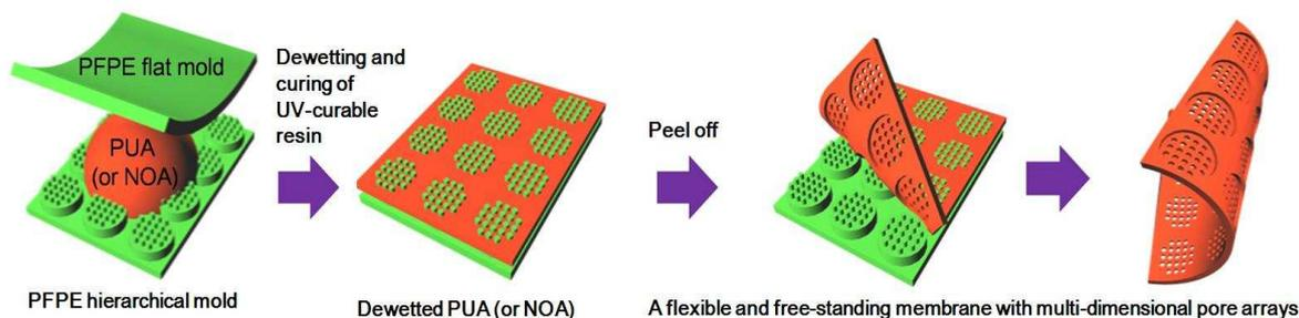
Figure 1. Dewetting-assisted fabrication of multi-dimensional pores on a polymeric hierarchical mold
