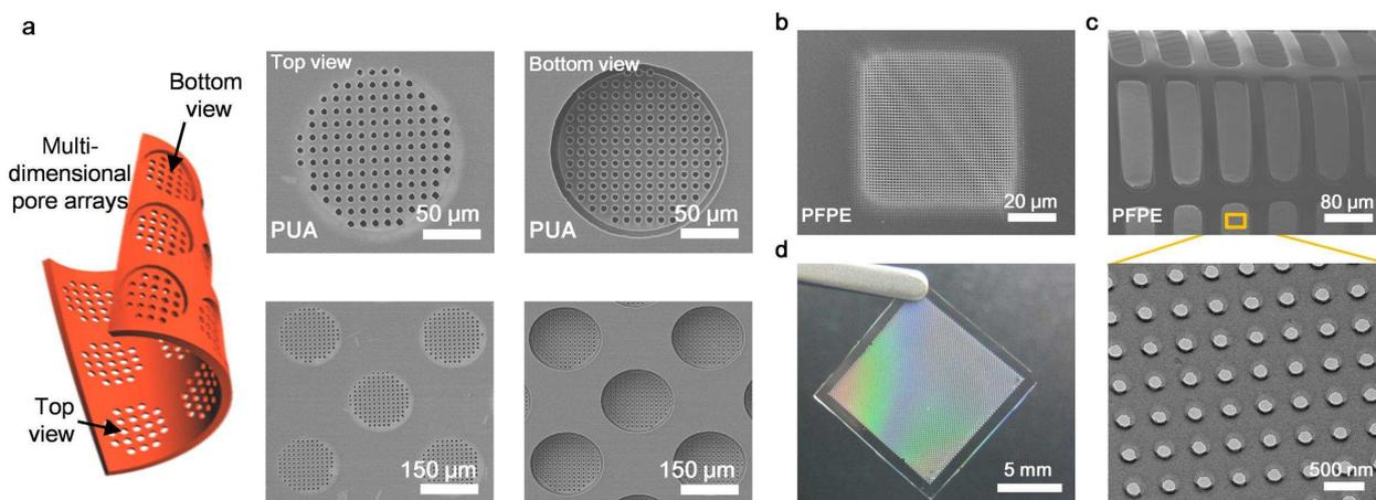
Figure 3. SEM and digital images of polymeric membranes with various sizes of multi-dimensional pores
