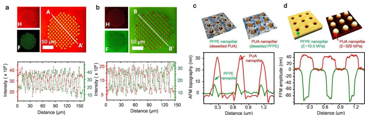
Figure 2. Chemical and mechanical mapping images of dewetting surfaces on hierarchical molds
