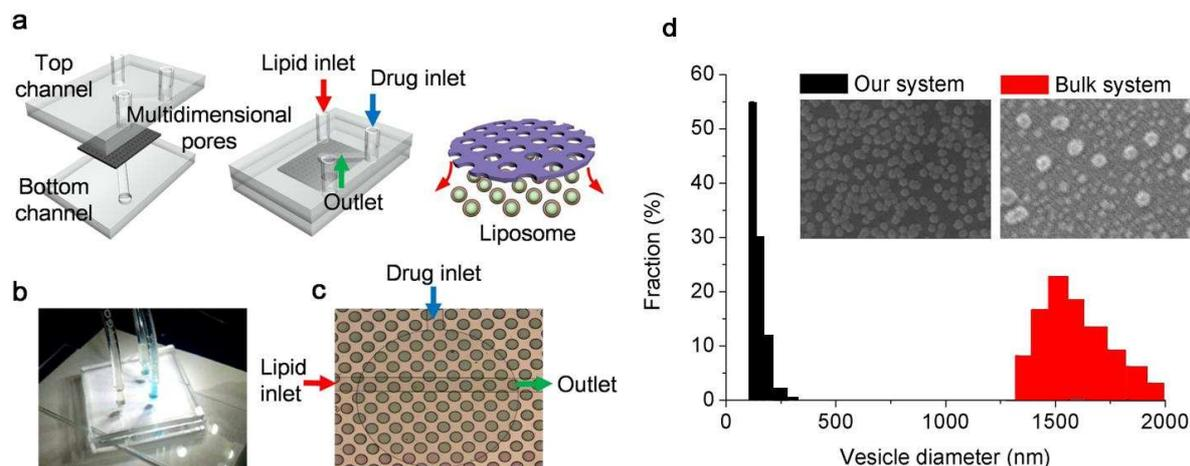
Figure 4. Schematic illustration of the synthesis of lipid vesicle in a microfluidic system with polymeric stencils
