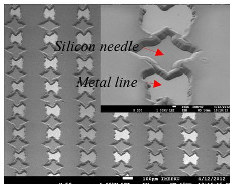
Figure 5: Backside of flexible MNEA
