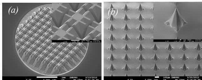
Figure 2: (a) diced silicon array; (b) Silicon microneedle array
