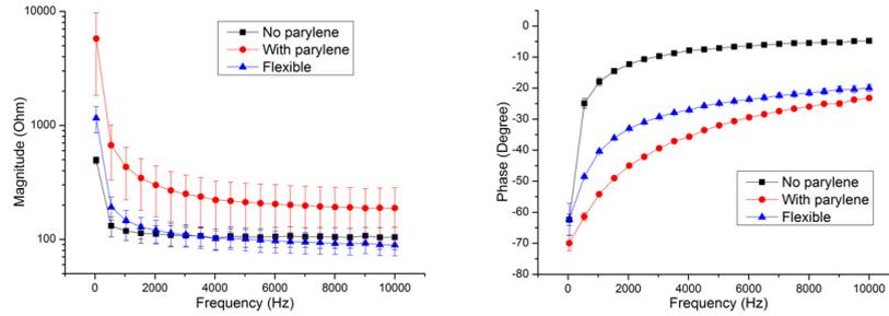
Figure 7: Impedances contrast of rigid and flexible MNEA
