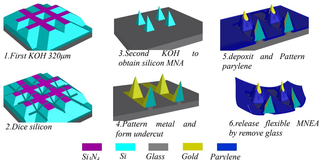
Figure 1: Schematic fabrication process
