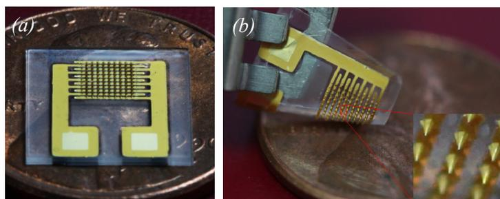
Figure 6: Photos of rigid and flexible MNEA: (a) Rigid MNEA with parylene; (b) Flexible MNEA
