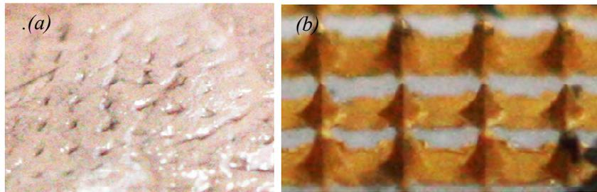
Figure 8: Penetration test of flexible MNEA:(a) spots indicated that flexible MNEA penetrated into tissue;(b)After penetration, MNEA retained previous structure and profile without obvious damage
