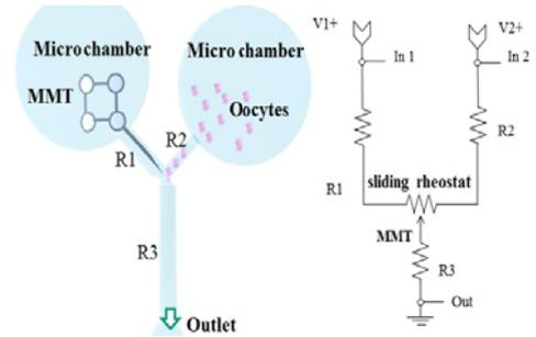
Fig. 2. The electric circuit analogy of the enucleation chip.
