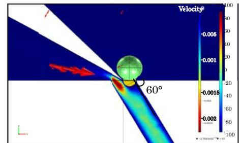
Fig. 4 FEM results of velocity distribution and the surface traction of oocyte.
