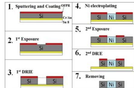
Fig. 5 Fabrication process of the MMT.
