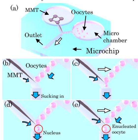
Fig. 1 (a) Overview of the enucleation microchip. (b-e) Oocyte enucleation process.
