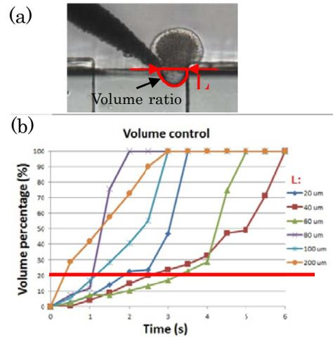
Fig. 3 Correlations of the volume sucked into the outlet microchannel and the time under the different displacement
