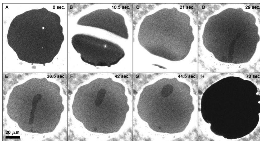
Figure 2. Confocal fluorescence images showing (a) lipid monolayer with air in the upper channel, (b, c) monolayer folding in progress, with lipid laden bubble-water interface clearly visible, (d) liquid ordered domains forming immediately upon completion of folding, with domain distortion resulting from shear forces during membrane formation, (e, f, g) domain recovery, and (h) induced bilayer rupture revealing low background fluorescence.
