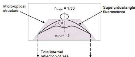
Figure 1: Principle of using the micro-optical structure for SAF emission detection.
