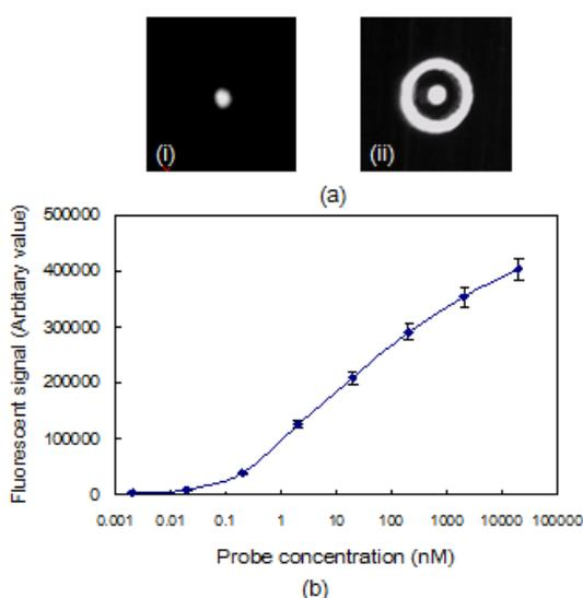
Figure 4. (a) Fluorescent images of DNA probe spotted on the micro-optical array. (b) Sensitivity test for the platform.
