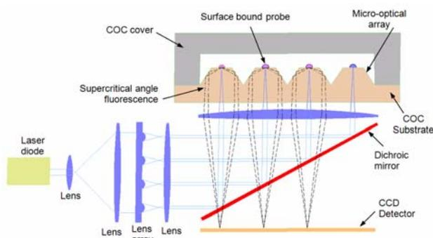
Figure 2. Schematic diagram of the detection platform.
