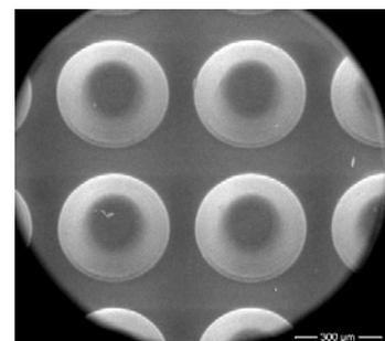
Figure 3. SEM of the micro-optical array in the COC chip.
