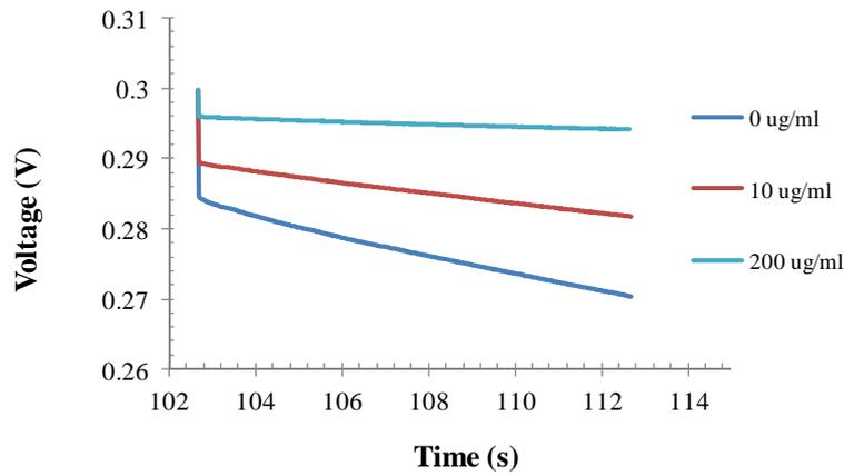
**Figure 5.** Dynamic voltage response of the IDA electrodes after the captured CRP was delivered to the electrodes from the immune-like biosensors.
