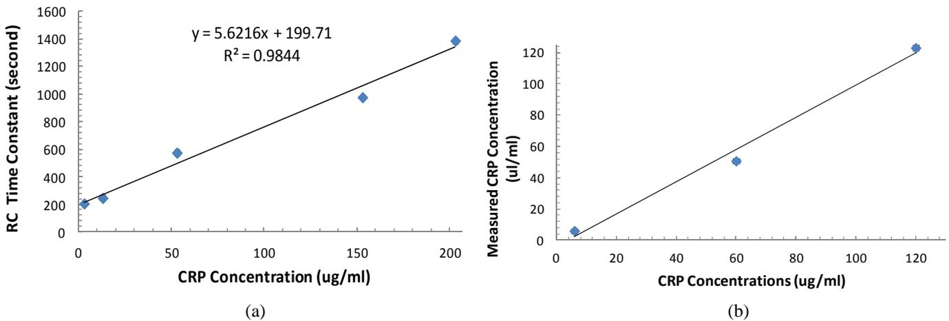
**Figure 6.** Measurement results of the developed biochips for rapid detection of CRP in human serum: (a) calibration curve and (b) the measured CRP concentrations according to the calibration curve.
