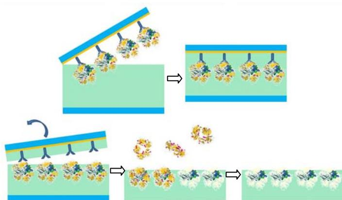
**Figure 2.** Fabrication process of the developed immune-like biosensors for CRP detection.
