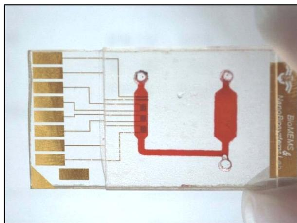
**Figure 3.** Photographs of the fabricated microfluidic biochip with on-chip immune-like biosensors.
