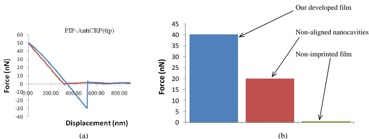
**Figure 4.** Characterization of the developed sensing films by AFM: (a) adhesion forces between our developed film and antibody and (b) comparisons of the adhesion forces caused by specific binding.
