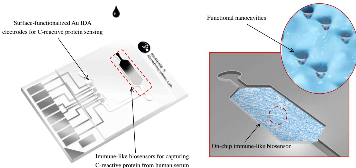
**Figure 1.** Schematic illustration of the developed electronic microfluidic biochips with on-chip immune-like biosensors for rapid detection of C-reactive protein in human serum.
