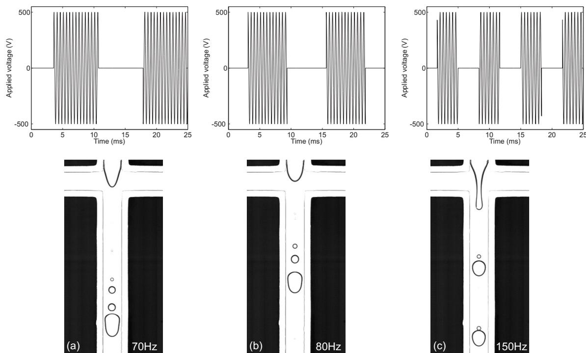
Figure 3: Controlled generation of different number of droplets. (a) 4 successive droplets, (b) 3 successive droplets and (c) 2 successive droplets. The droplets are generated at fixed flow rates of 250:75:250  $\mu\text{l/hr}$  and the droplet production frequency is about 140 Hz. For clarity, the displayed frequency (top figures) is 2 kHz (50 kHz in experiments).
