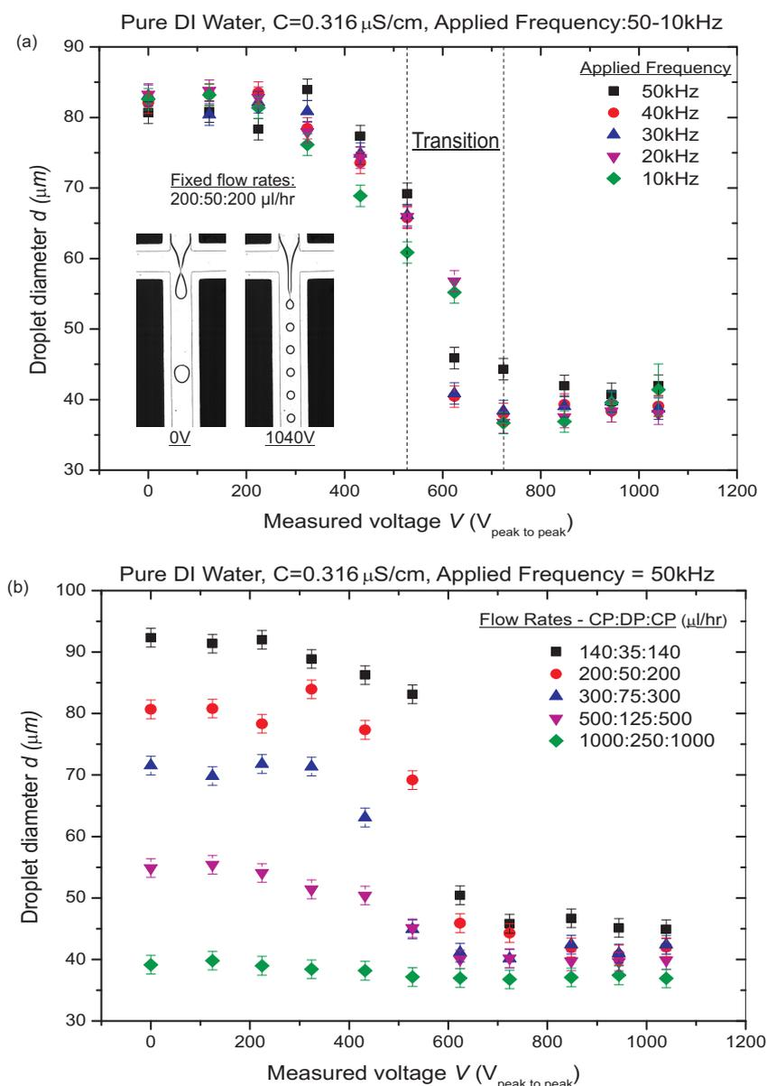
Figure 2(a) Effect of different applied frequency. (b) Effect of using different total flow rates at a fixed ratio of 8. In both experiments, alternating voltages (sinusoidal wave) are applied to the top pair of electrodes while the bottom pair of electrodes and the ITO plate is grounded.
