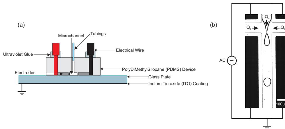
Figure 1: (a) Schematic sketch of the microfluidic device used. (b) Optical image of the geometry used.
