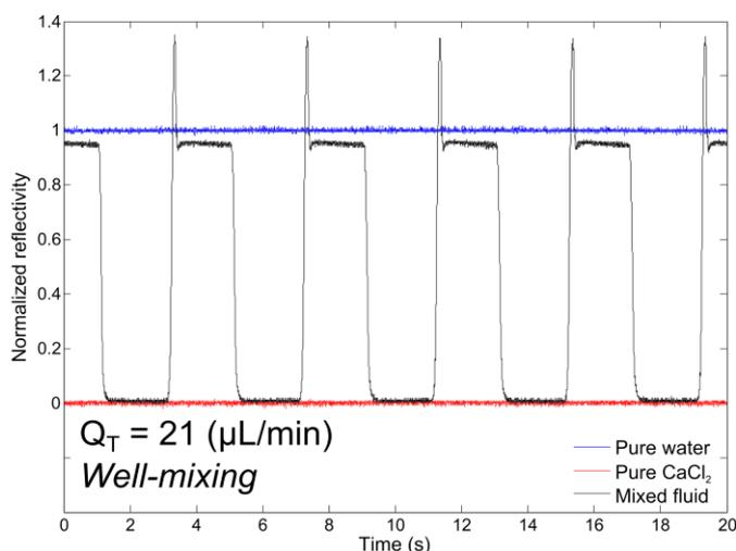
Figure 3: The normalized signal waveforms under  $Q_T = 21 \mu\text{l}/\text{min}$  ( $Q_T = Q_1 + Q_2$ ).
