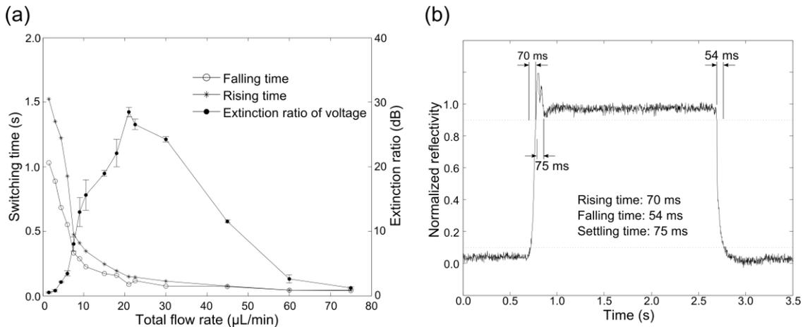
Figure 4: (a) Switching performance in response to total flow rate. (b) Analysis of the dynamic response of the device.
