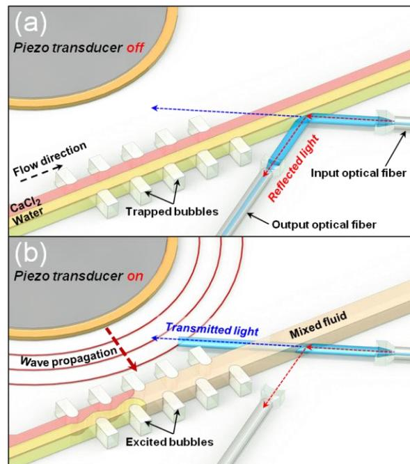
Figure 1: A schematic showing the design and working principle of the acoustofluidic optical switch.
