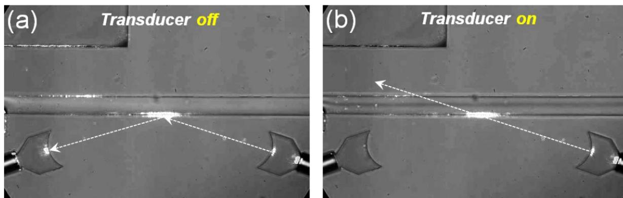
Figure 2: Experimental images of the optical switch. (a) The device without acoustic excitation. (b) The device under acoustic excitation. The dotted arrow represents the light path.
