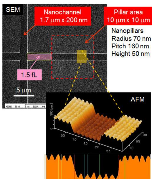
Figure 2. AFM image of fabricated nanopillar-in-nanochannels
