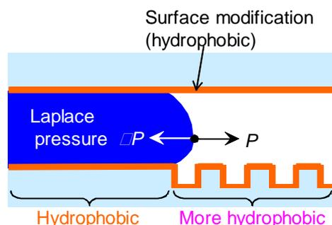
Figure 1. Concept of nano Laplace valve by nanopillar-in-nanochannel and surface modification
