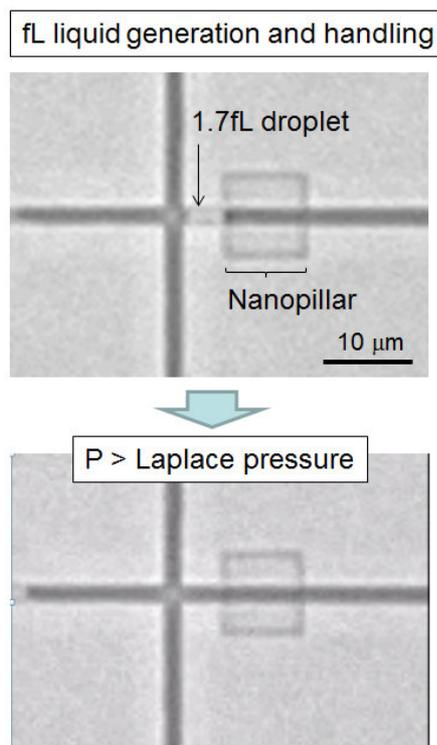
Figure 5. 1.7fL droplet generated in air (upper) and shot of the droplet by applying higher pressure than Laplace pressure
