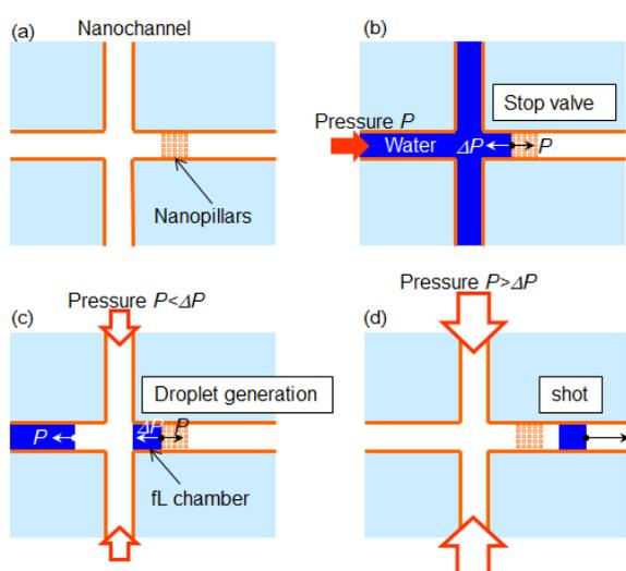
Figure 4. Procedures for fL liquid generation in air and shot.
