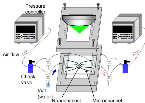
Figure 3. Pressure-driven liquid handling system and microchip
