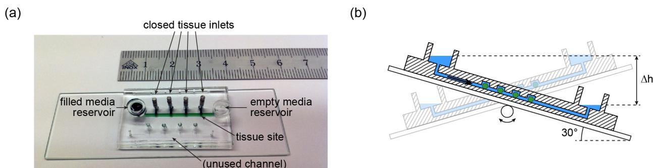
Figure 2: (a) Photograph of the PDMS chip, loaded with green food dye for visualization. The tissue inlets have been closed with stainless steel pins after loading. Two media reservoirs are used for perfusion. The flow-rate is controlled by automated tilting of the device at specific angles generating a hydrostatic pressure difference between the two media reservoirs (b).
