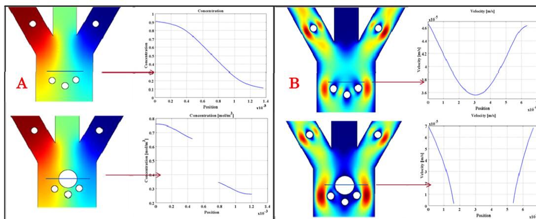
Figure 2 Simulation of chemical gradients (A) and flowing velocity (B) in the -device with or without EB by Comsol Multiphysics. When two kinds of chemical solutions are perfused into the device, Figures on the right show the chemical gradient (or flowing velocity) along the blue line in the left pictures. It indicated that a proper chemical gradient existed at the crossing (B) and flowing velocity was the least there (B).
