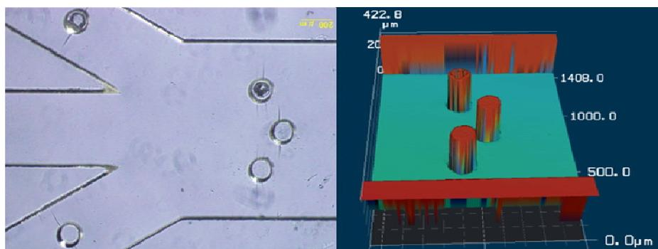
Figure 1 Two dimensional and three dimensional structures (by laser microscope) microphotographs of the microfluidic device; PDMS pillars (dia.80 $\mu\text{m}$ , height, 430 $\mu\text{m}$ ) standing at the crossing or channel for preventing from EB washing away;
