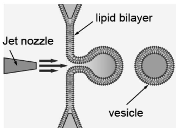
**Fig.1** Illustration of cell-sized vesicle formation from planar lipid bilayer using pulsed jet flow.
