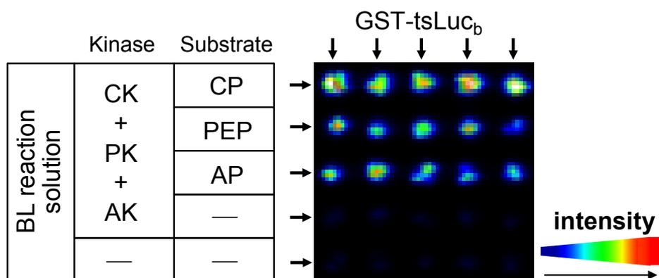
Fig. 3. CCD image of the on-chip BL in simultaneous assay for kinases. CK; creatine kinase, PK; pyruvate kinase, AK; acetate kinase, CP; creatine phosphate, PEP; phosphoenolpyruvate, AP; acetyl phosphate.
