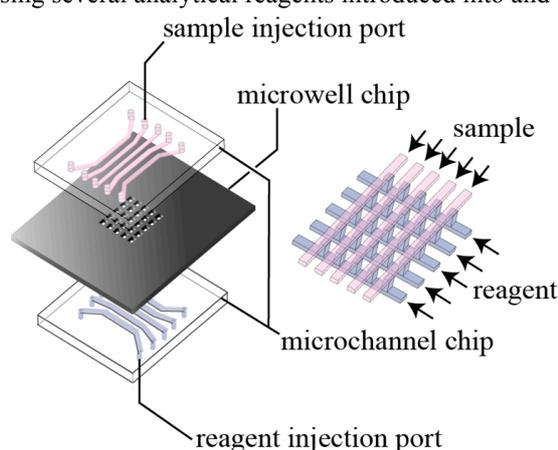
Fig. 1. Schematic of the on-chip assay system.
