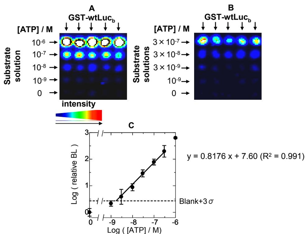
Fig. 2. CCD images of the on-chip BL at various concentrations of ATP (A and B), and calibration curve for ATP (C).
