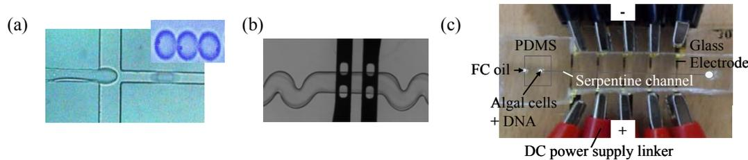
Figure 2. Algal cell electroporation on microfluidic chip: optical image of (a) droplet generation and single cell encapsulated in a droplet, (b) serpentine channel and electrode, and (c) whole electroporation chip system. The scale bar is 50  $\mu\text{m}$
