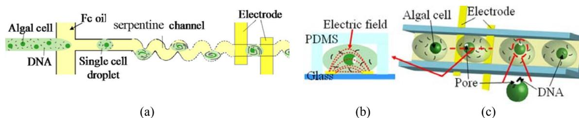
Figure 1. Principle of droplet microfluidic electroporation (a) schematic diagram, (b) a droplet with cell over electrode, and (c) electroporetic process of algal cell
