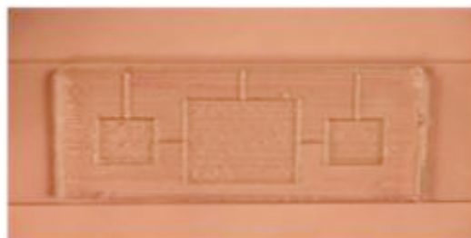
Fig. Top view of PDMS chip comprises of inlet reservoir, outlet reservoir, one main chamber and microchannels
