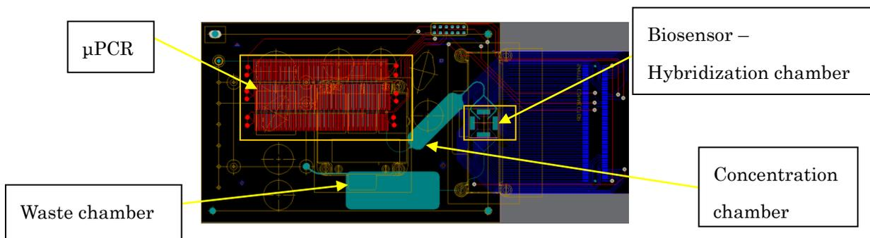
**Figure 3.** Complete design of all LoC layers
