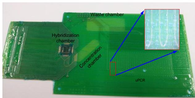
**Figure. 5** Fabricated microchannels.
