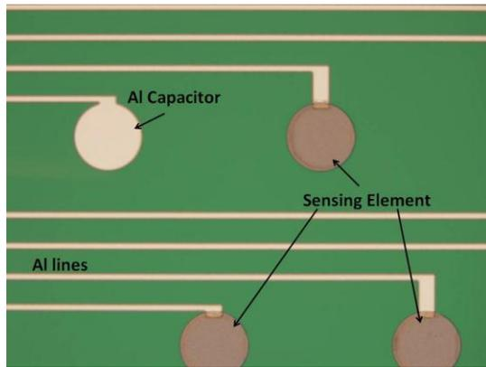
**Figure. 1** Image of part of the sensor array consisting of membranes (sensing elements) and an Al capacitor.
