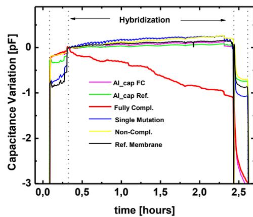
**Figure. 2** The average response of several sensing elements during DNA hybridization of 15mer model oligos.
