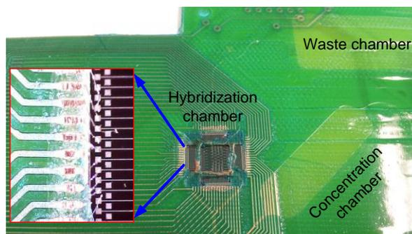
**Figure. 6** Hybridization chamber with biosensor chip wire bonded to the Cu pads of the PCB to provide electrical connections.
