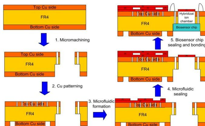
**Figure 4.** LoC fabrication process flow
