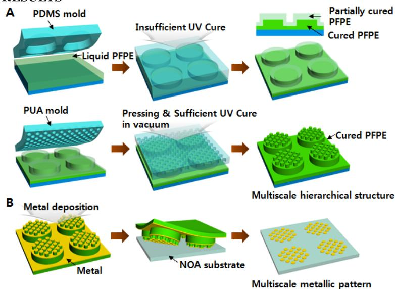
Figure 1. Fabrication of multiscale metallic patterns using a hierarchical stamp
