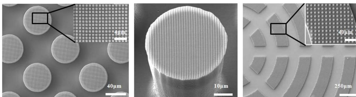
Figure 3. SEM images showing examples of hierarchical structures with various shapes and scales
