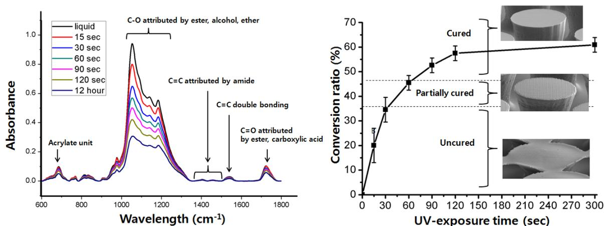
Figure 2. FT-IR spectra and conversion ratio of PFPE below the PDMS mold depends on the UV exposure time.
