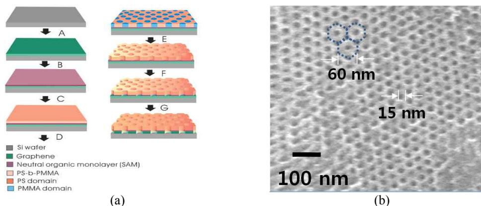
Figure 1. Schematic diagram of the graphene nanosieve using block copolymer lithography process (a), and the SEM photograph of graphene sieve with nanopores of a diameter of 15 nm (b).
