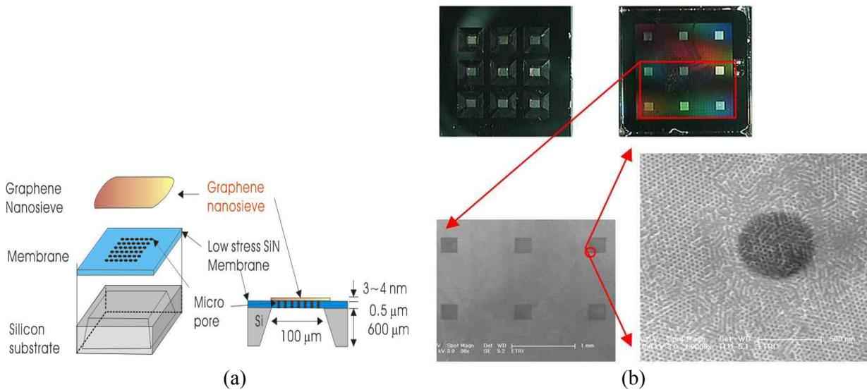
Figure 2. Cross-sectional view of the nano-sieve devices; top and bottom photographs(a) and top SEM photographs of them (b).
