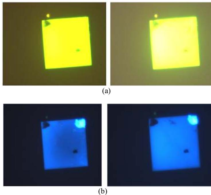
Figure 3. Fluorescence photographs showing selective penetration of mixture of two proteins (Hb) (a) and Immunoglobulin G (IgG) (b) at separation-starting time and after 10 min. IgG is tagged with 350 nm-fluorescence dyes and Hb with 480 nm-fluorescence dye.
