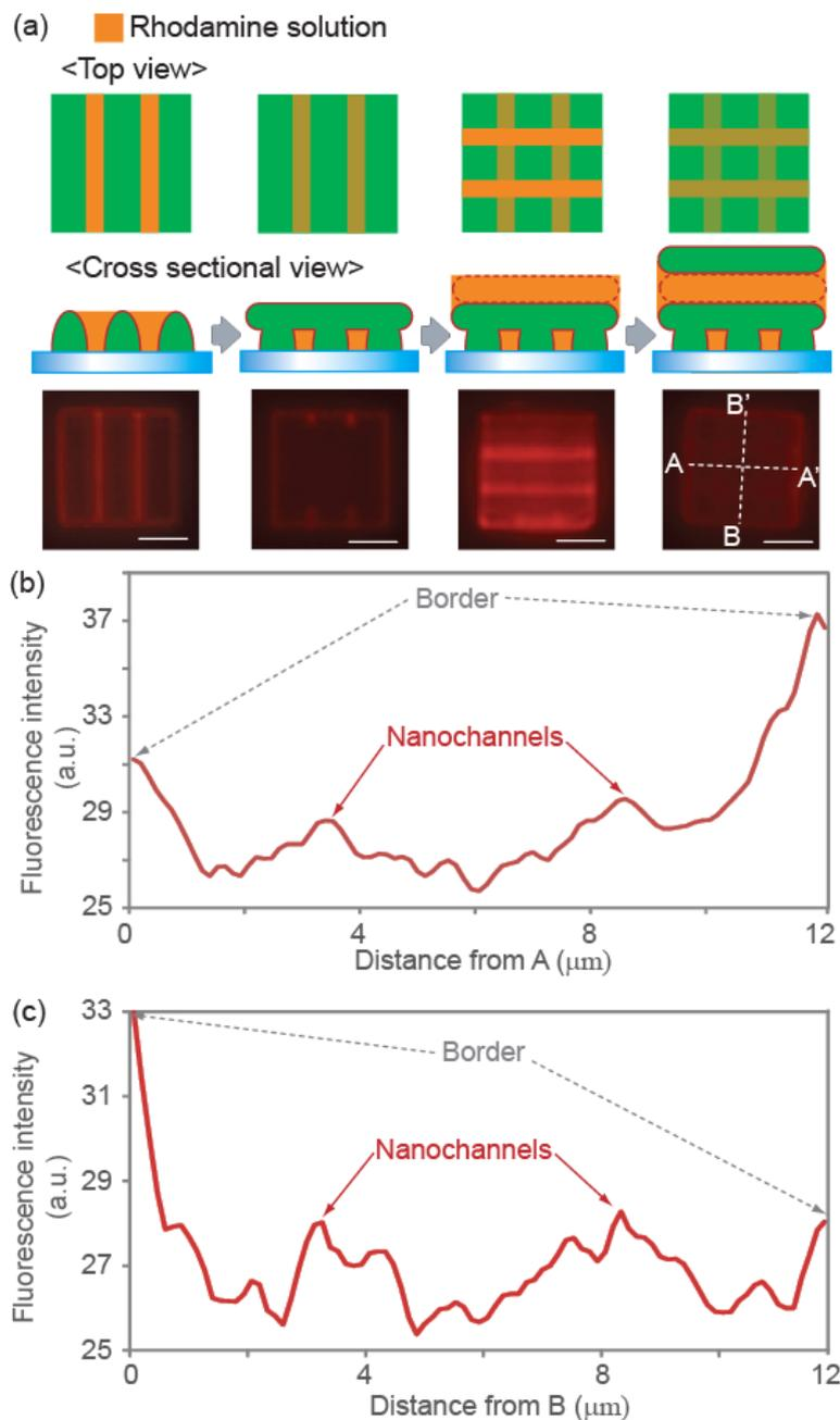
Figure 4. Vertical array of nanochannels. (a) Vertical array of nanochannels fabricated by laser-writing process in Fig. 2. The dye solution could flow into the nanochannels. Scale bars indicate 5  $\mu\text{m}$ . Fluorescence intensity along line (b) AA' and (c) BB'. 4 nanochannels in the vertical array could flow the dye solution. The border of the structures glowed due to dye absorption.
