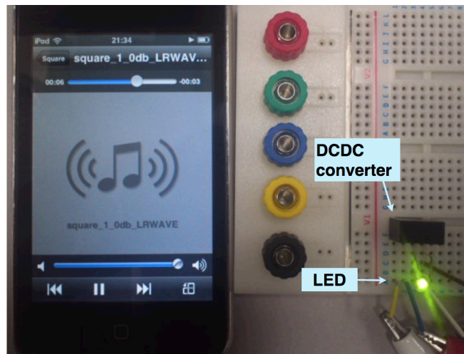
Figure 4. An activation of a green LED by our system with an DC-TO-DC boost converter.
