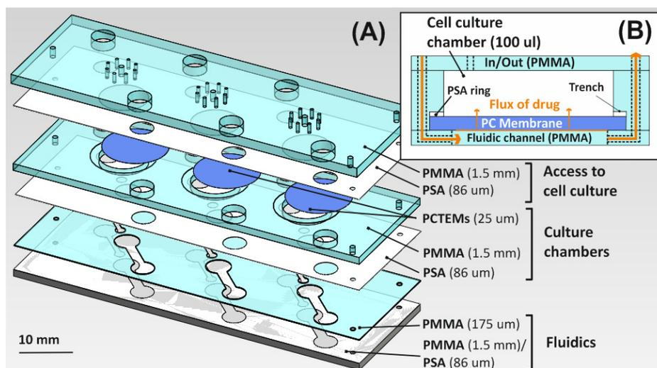
Figure 1: 3D schematic of the device assembly (A) and cross sectional view (B). The device consists of three main compartments: (i) fluidic structures defined in the bottom PMMA/PSA layer, (ii) PMMA culture chambers with integrated GE Whatman<sup>®</sup> polycarbonate track-etched membranes installed on PSA rings and (iii) a PMMA cap with inlets to introduce cell culture and gaps to supply sufficient aeration of cells.
