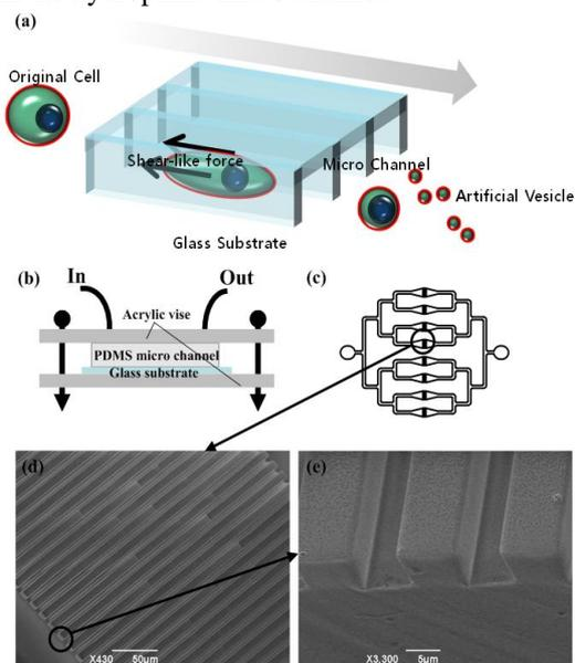
Figure 2. (a) Diagram showing generation of artificial-nano-vesicle using a simple micro channel. (d), (e) Scanning Electron Microscopic Images of extrusion channels.
