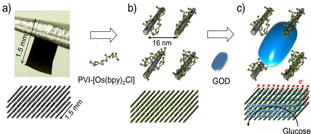
Figure 1. Photograph and schematic illustration of the CNTF-based glucose oxidation electrode prepared by stepwise modifications of PVI-[Os(bpy)<sub>2</sub>Cl] and GOD inside a CNTF film.
