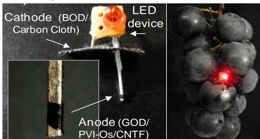
Figure 3 (Left) Photograph of the LED-based self-powered sugar indicator, at the tip of which the GOD/PVI-[Os(bby)<sub>2</sub>Cl]/CNTF film was wound. (Right) The device assembly was inserted in a grape to measure the LED blinking interval that correlates with the glucose concentration.
