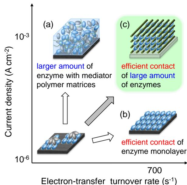
Figure 4. Scheme showing correlative characters of (a) an enzyme-film with mediator polymer matrices for larger current, (b) an enzyme-monolayer electrode for higher turnover rate, and (c) the present ensemble electrode for both large current and high turnover rate.
