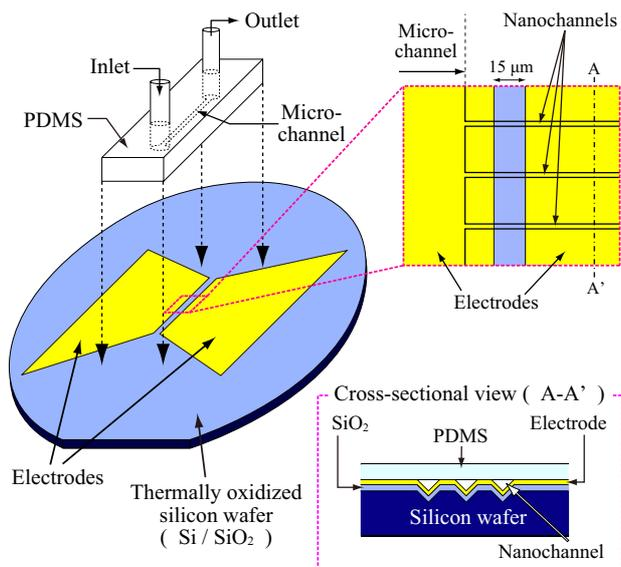
Figure 2. Schematic of a micro/nano fluidic device for nanowire formation.
