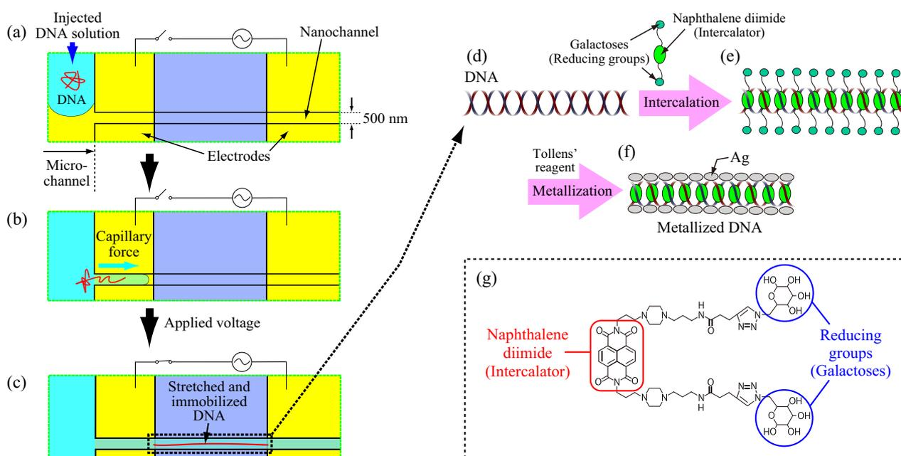
Figure 1. Procedure of formation of a single metallized DNA nanowire (a-f) and structural formula of reducing group-labeled intercalator (g).
