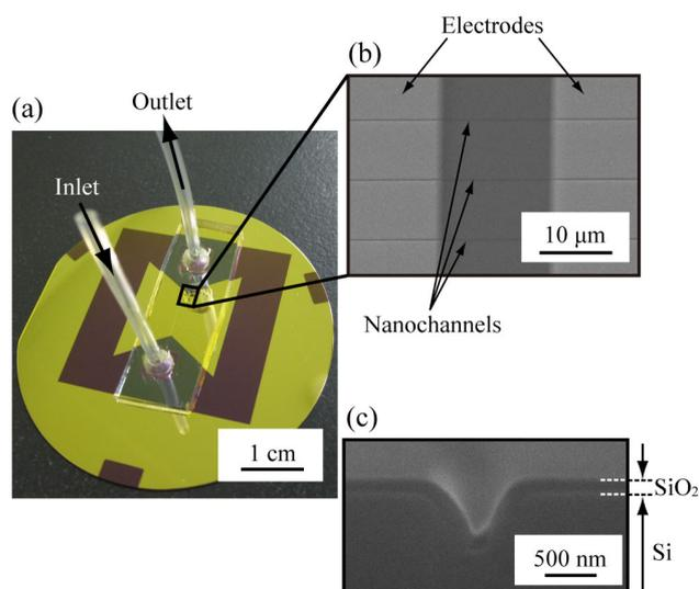
Figure 3. Photographs of the fabricated device and SEM image of the nanochannel.
