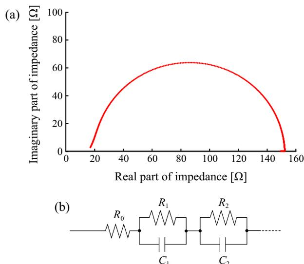
Figure 7. Complex impedance plot and an equivalent circuit of the metallized  $\lambda$ DNA nanowire.
