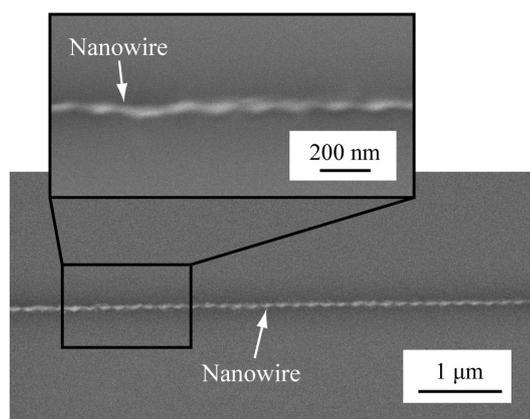
Figure 5. SEM images of the metallized  $\lambda$ DNA nanowire.
