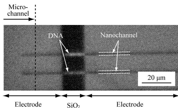
Figure 4. Fluorescence image of the  $\lambda$ DNA stretched and immobilized between the electrodes.
