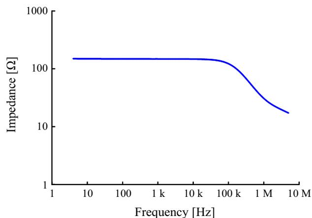
Figure 6. Impedance spectrum of the metallized  $\lambda$ DNA nanowire.
