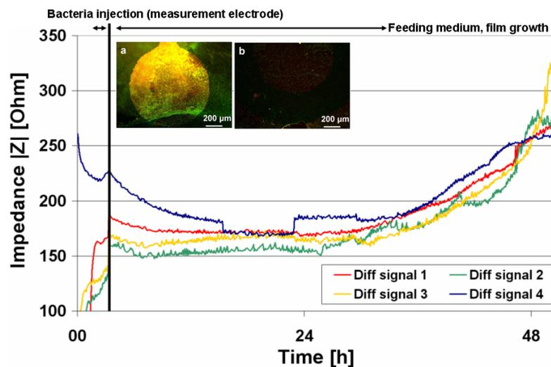
Figure 4 - Differential impedance measurement. During the first 3 hours of the experiment the measurement electrode was probed with *Staphylococcus aureus*, followed by feeding medium. Reference electrode only came in contact with feeding medium. After 48 hours the results tend to be affected by air bubbles. The inlay pictures show the live-dead staining of these electrodes. a) Measurement electrode b) Reference electrode.
