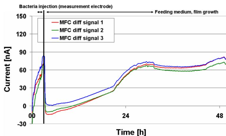
Figure 5 - Differential current measurement over 48 hours of the MFC electrodes. An increase in the signal can be observed which correlates to the increase in measured impedance.
