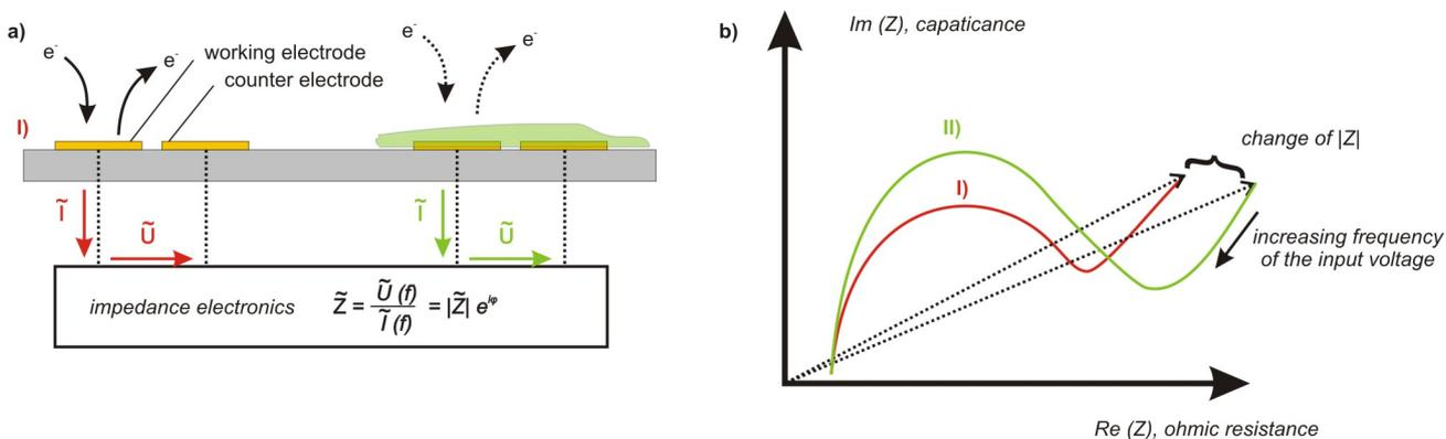
Figure 1 - a) Principal setup of EIS in biofilm detection – to a pair of electrodes a small AC voltage is applied and the current between the electrodes is measured. b) The impedance is usually displayed in the complex plane in form of a Nyquist diagram (displaying real and imaginary parts of the complex resistance).
