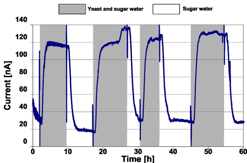
Figure 3 - Microbial fuel cell (MFC) activity sensor test in a yeast and sugar water microreactor. Gray shaded intervals mark the injection of yeast and sugar water. During other intervals only sugar water was probed across the sensor. The switching of the pump is responsible for the presence of peaks in the diagram.
