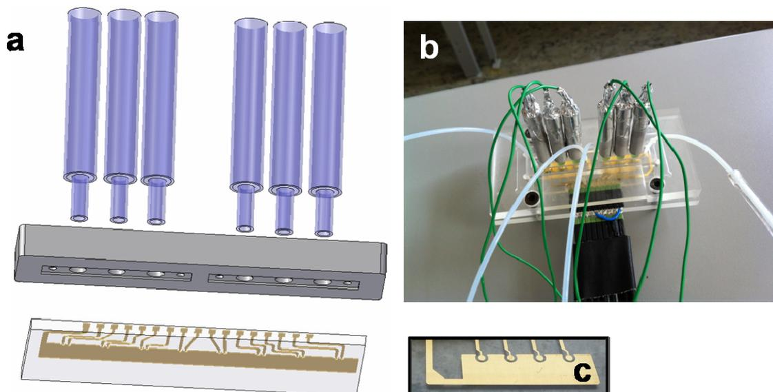
Figure 2 - View of the flow cell setup. a) Schematic view of flow cell, MFC activity sensors on the top, flow cell in the middle and planar electrodes at the bottom. b) Picture of the measurement cell. c) EIS planar electrode.
