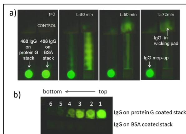
Figure 3: a) Time-lapse images of Alexa 488 labeled IgG flowing through the protein G-coated membrane stack in the 2DPN assay card. A BSA-coated membrane stack was used as a control. Arrows indicate successful IgG removal by the protein G-coated stack, whereas in the control, IgG collects in the wicking pad. b) Individual membranes from the protein G and BSA-coated membrane stacks indicate labeled IgG levels in each case.
