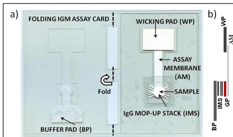
Figure 2: a) Foldable 2DPN IgM assay card with a stack of six nitrocellulose membranes coated with protein G for IgG “mop-up” overlaying the assay membrane via secondary gold label pad (GP). The assay is operated by adding sample over the topmost layer of the stack and folding the card to bring the buffer pad in contact with the stack. b) Side-view of the layers.
