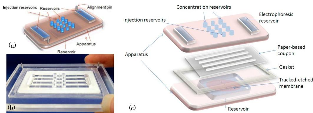
Figure 1: (a) Schematic of pre-concentration/electrophoresis floupon system (b) A photograph of the electrophoresis apparatus (c) Schematic of the layers of pre-concentration/electrophoresis system.
