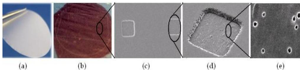
Figure 2: (a) Image of tracked-etched membrane prior to patterning (b) Patterned membrane with Shipley resist coating (c) SEM image of patterned membrane where the openings are patterned using photolithography. (d) SEM image of one of the openings in the membrane (e) SEM image of the 15 nm pores inside the opening in the membrane
