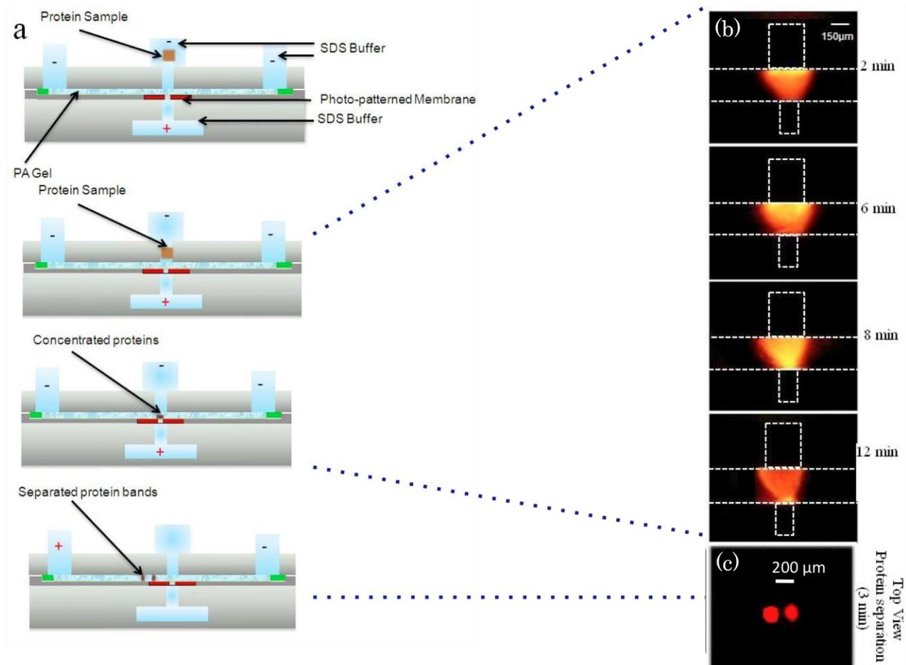
Figure 3: (a) Schematic Side view of pre-concentration apparatus. Photo-patterned membrane allows the concentration of proteins by trapping the proteins on the membrane while allowing electric field line to pass through goat anti-rabbit (c) Top view image of goat anti-rabbit Alexa flour 532 antibody after 3 minutes of separation into heavy and light chain.
