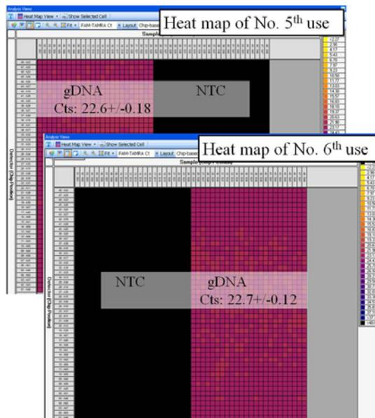
Figure 4. Two real-time PCR Ct heat maps in continuous use of same reusable array. In the following cycling, the right half of chip, which was loaded with positive reactions, has shown successfully recovered from previous use. And the left half of chip, which was loaded negative reactions, has demonstrated no amplicon carryover from previous chip run.
