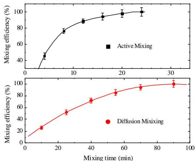
Figure 2. Mixing efficiency changes versus mixing time
