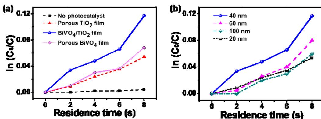
Figure 3 (a) The photocatalytic performance of the microreactor using BiVO<sub>4</sub>/TiO<sub>2</sub> film as compared to the other control experiments; (b) influence of the BiVO<sub>4</sub> film thickness.
