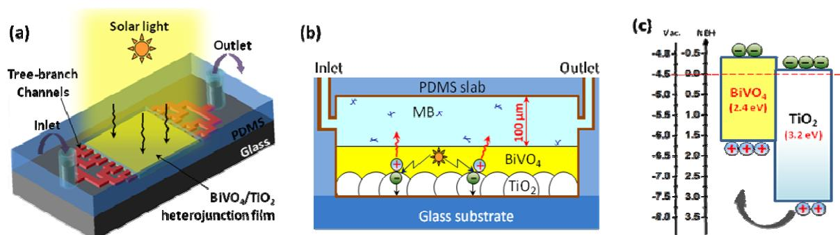
Figure 1: Design and working principle of the microreactor. (a) 3D schematic of the microreactor structure; (b) cross-sectional view of the reaction chamber; and (c) Energy band diagram of  $\text{BiVO}_4/\text{TiO}_2$  heterojunction film.
