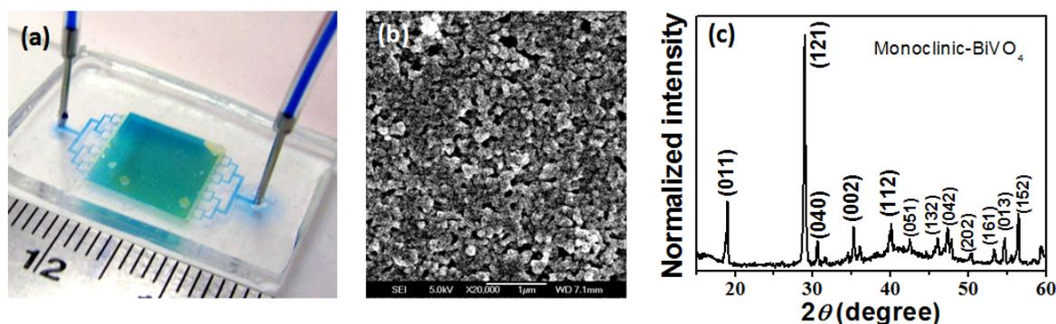
Figure 2: (a) Photograph of the microreactor; (b) scanning electron micrograph of the compound BiVO<sub>4</sub>/TiO<sub>2</sub> film; and (c) XRD of the BiVO<sub>4</sub> deposited by PLD, showing the monoclinic phase.
