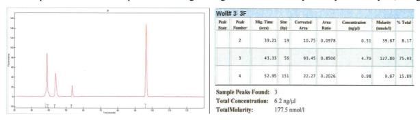
Figure 3 Result of an analysis of a PCR amplicon using the LOC system by Bioanalyzer (above). High DNA concentration of the amplified PCR product of 4.7ng/µl was archived (right).
