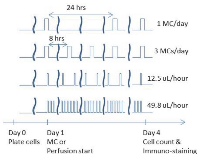
Figure 2: Schematics of medium change protocols under static culture and perfusion culture. hiPSCs were loaded at day 0 and placed to adhere in microchamber for overnight. From day 1 after plating, medium were changed with one medium change per day (1 MC/day) and three medium changes per day (3 MCs/day), or perfused at indicated flow rate.
