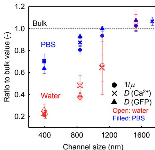
Figure 6 Diffusion coefficients  $D$  compared with inverse of the viscosities  $1/\mu$  to verify the Stokes-Einstein relation. Parameters are normalized by that in the bulk.
