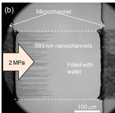
Figure 2. (a) Schematic of experimental setup for observation of capillary flow in extended nanochannels driven by high pressure control system. (b) Image of capillary flow driven by external pressure of 2 MPa.
