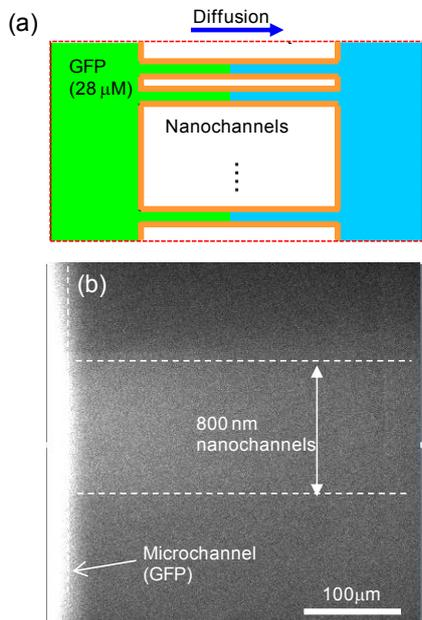
Figure 3 (a) Schematic of diffusion of GFP through extended nanochannels. (b) Image of diffusion of GFP (28  $\mu\text{M}$ ) in nanochannels.
