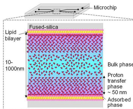
Figure 1. Schematic of bio-mimetic extended nanospace, where fused-silica extended nanochannel is modified by lipid bilayer.
