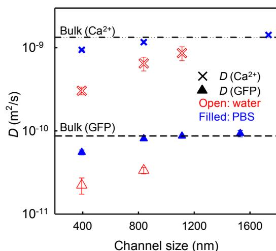
Figure 5 Diffusion coefficients as function of the size of bio-mimetic extended nanochannels.
