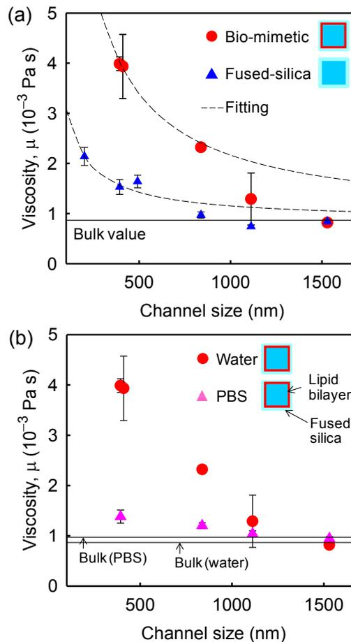
Figure 4 (a) Water viscosity as function of the size of bio-mimetic- and fused-silica extended nanochannels. (b) The viscosity of PBS and water in bio-mimetic extended nanochannels as function of the channel size.
