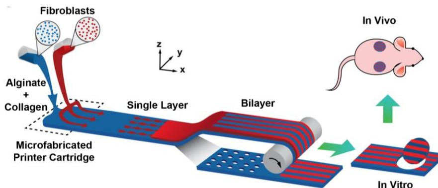
Figure 2: Illustration of proposed skin printer for formation of cell-populated skin substitute in a microfabricated printer cartridge and application in vivo.
