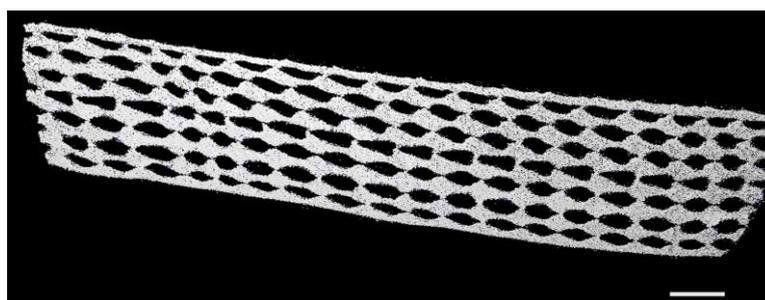
Figure 4: Microcomputed tomographic scan of patterned planar sheet containing a hole array. Contrast obtained by incorporating 1%w.t.  $\text{BaSO}_4$  into the biopolymer sheet solution. Scale bar 1mm.
