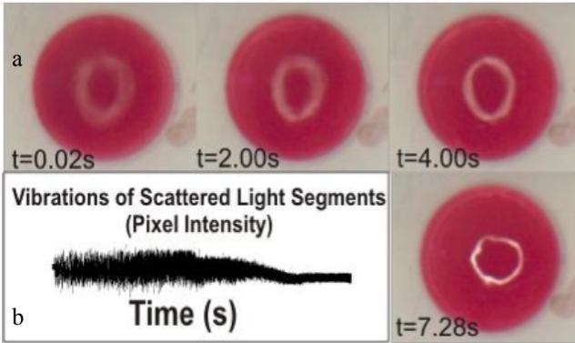
Figure 3: (a) Effect of SAW on a 4-μl blood drop at various times after the actuation. The streaming induces high shear rates in the drop, causing the red blood cells (RBCs) to aggregate together resulting in the blood having an increased viscosity locally. (b) A cross-section of a line passing through all the 364 images (7.28 s) of solidification process was observed by a YZ orthogonal stack of the scattered light ring in time domain.
