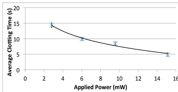
Figure 6: Time taken for a 4 $\mu$ l droplet at 8.83Mhz to achieve equilibrium (as described in Fig 3&4) for different input powers (2.8-15.1 mW). As the power increases, the solidification becomes faster, reaching ca 5s at 15.1 mW.
