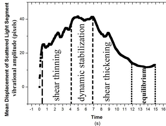
Figure 4: Shows the mean displacement of scattered light segment that was obtained from calculating the average width of each frame of scattered light segment acquired from Fig 3(b). The vibrations indicate blood viscoelastic behavior changing from initial shear thinning as the displacement becomes larger over a similar period of time, to shear-thickening, when the displacement reduces and finally solidifying. A 4μl droplet at 8.83Mhz, 15.13 mW input power was used.
