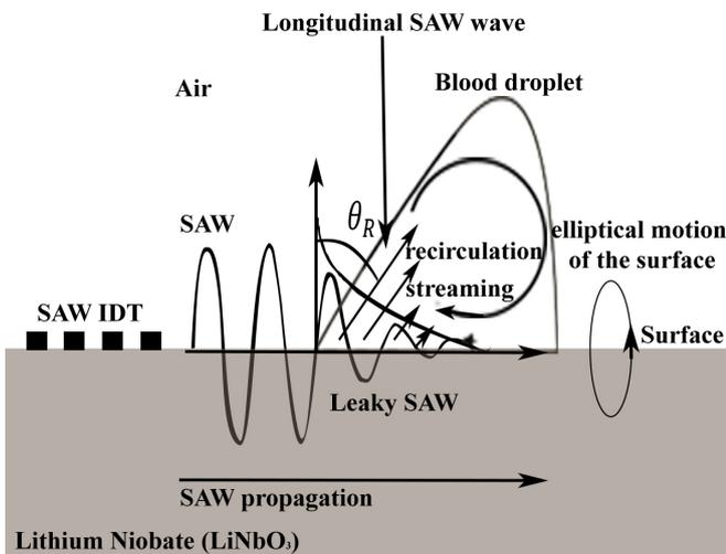
Figure 1: Interaction of SAW interaction with a fluid leads to acoustic streaming flows and a longitudinal pressure wave in the fluid.
