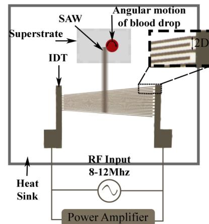
Figure 2: Schematic of a slanted IDT and the SAW propagating into blood causing streaming. An Agilent Technologies MXG Analog Signal Generator N5181A was used in conjunction with a Mini Circuits ZHL-5W-1, 5–500 MHz amplifier with a gain of 38 dBm to actuate the SAW device. The piezoelectric surface was coupled with a heat sink to control the temperature.
