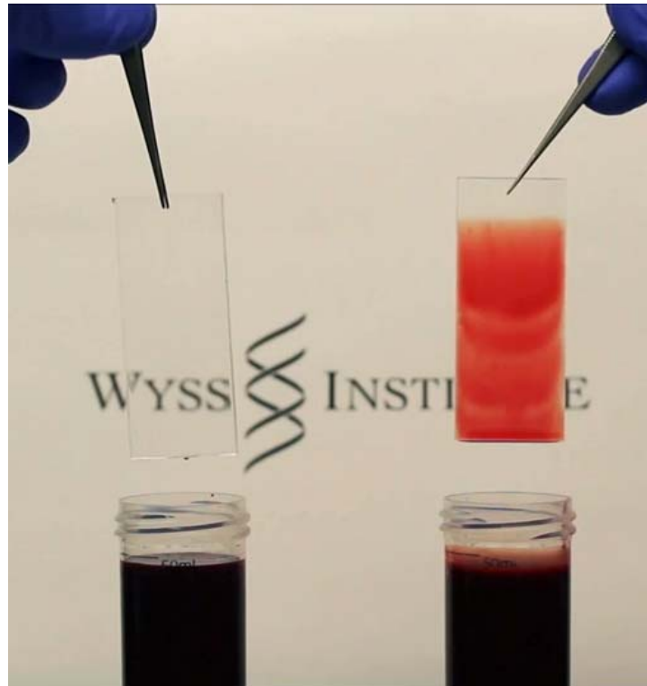
Figure 1: TLP-coated surfaces repel whole human blood. Tethered liquid perfluorocarbon (TLP) surfaces (left) showing the tethered perfluorocarbon (TP) bound to a substrate through plasma activation and silane treatment, which allows a stable film of liquid perfluorocarbon (LP) to adhere to the surface. When both the tethered and liquid perfluorocarbons are applied to the surface, TLP, the acrylic surface resists the adhesion of whole human blood even after complete immersion (left side). Surfaces without the tethered or liquid perfluorocarbon (-TP/-LP) show substantial adhesion of a blood after immersion in blood over 5 seconds (Control, right).
