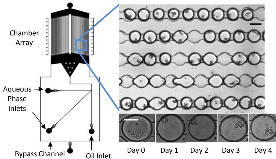
Figure 2: (Left) Diagram of the microfluidic device used for spheroid formation within droplets and their on-chip storage. (Right) Brightfield image of M/O droplets containing spheroids stored within the chamber array (top right image scale bar = 230  $\mu\text{m}$  and bottom left scale bar = 115  $\mu\text{m}$ ).
